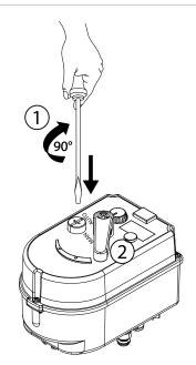
1) With a screwdriver push and turn off the button to the MAN position
